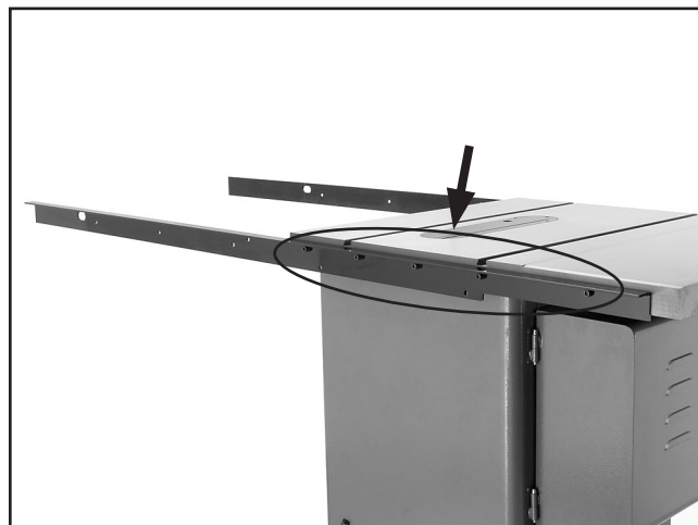
Figure 11. Rear rail installed.
